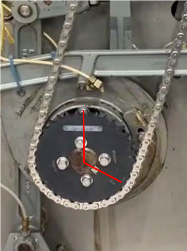
Sprocket key is at 135 degrees.
