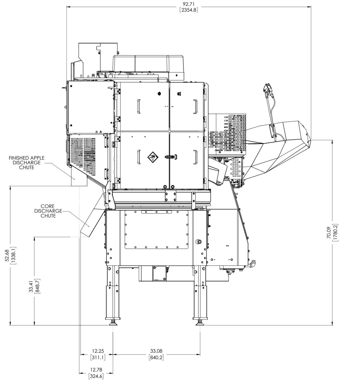
1. THE LEG HEIGHT CAN BE ADJUSTD PLUS OR MINUS 2" [50.8] FROM THE DIMENSIONS SHOWN.
